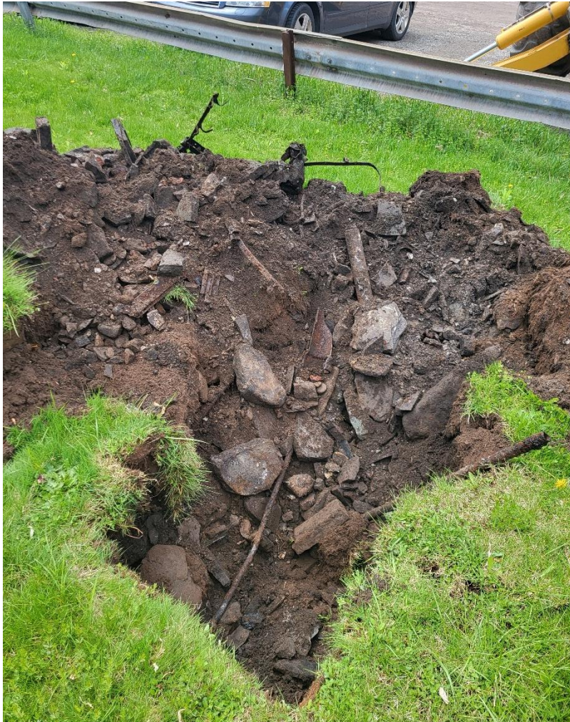
Figure 2: Stone foundation, construction debris, and burnt rubble from former building in Test Pit #2.
