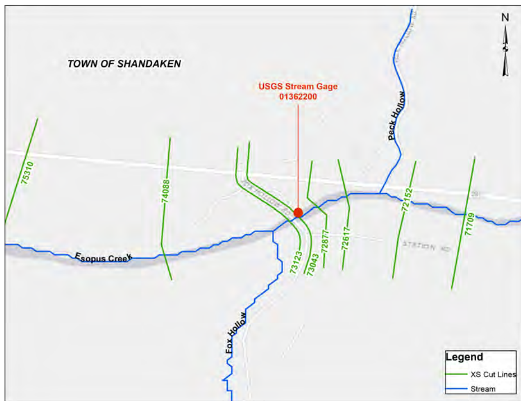
Figure 1. Esopus Creek HEC-RAS model in the vicinity of USGS stream gage 01362200.
